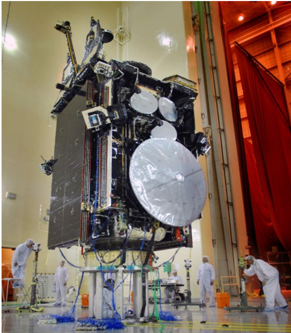
Military COMSAT after Environmental Testing [1]
